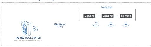
\*Wireless repeater is recommended for areas with poor signal reception
