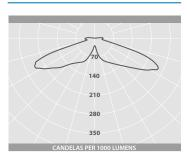
Luminaire Lumen Output: 31W = 4320lm 52W = 6825lm
